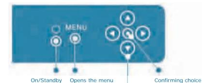
Up/down arrowkeys for navigation within the menu. If the menu is closed they work as Prog-and Prog+Left/right arrowkeys for navigation within the menu. If the menu is closed they work as Vol- and Vol+
