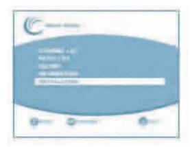
Click the SETUP button on your remote control Highlight the INSTALLATION menu option Press the OK button and you will be brought to the following menu:
