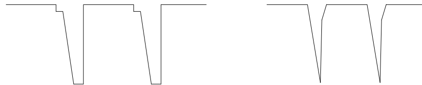
- normal wave form - - unnormal wave form - figure 7-4-3. Q1 switching voltage wave form
