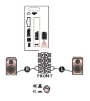
For improved sound, you can connect 2 external L and R loudspeakers in the place of the left and right loudspeakers on the TV set.
