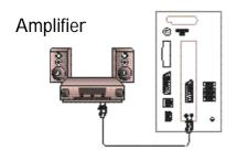
To connect to a hi-fi system, use an audio connection cable and connect the "L" and "R" outputs on the TV set to the "AUDIO IN" "L" and "R" input on your hi-fi amplifier.
