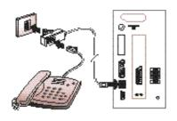
Your television is equiped with an integrated modem for digital information transfer via your telephone line. Connect a telephone cable as illustrated opposite.
